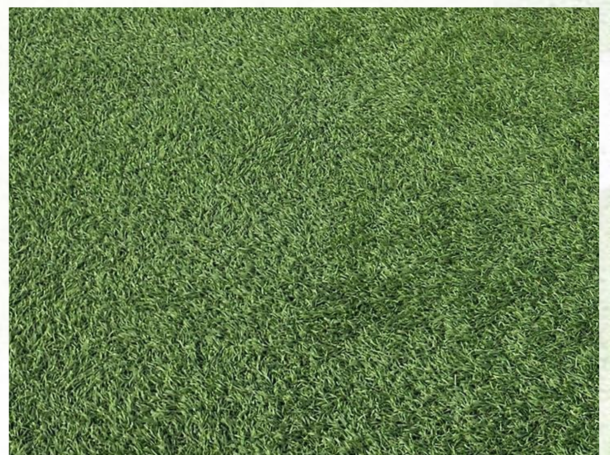
Example of an out-of-use pitch with irretrievably flattened fibres
